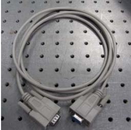
Chiller to Controller Cable
