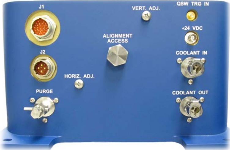
Figure 4-5 Connectors on the Rear Panel of the Gigashot™ Laser
