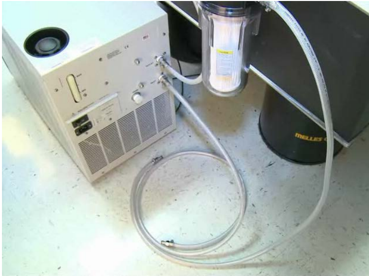
Figure 4-4 Chiller Assembled with Coolant Hoses and Filter
