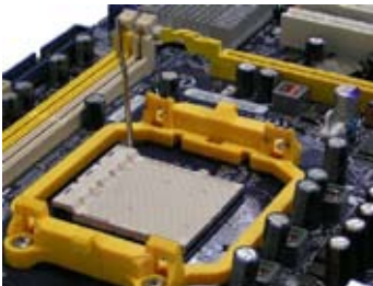
1. Release the CPU socket lever.
