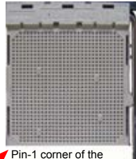
Pin-1 corner of the CPU socket
