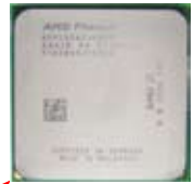
Pin-1 triangle marking of CPU
