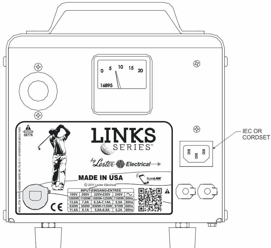
Figure 9.2-1: Links Series Model 2770 User Interface
