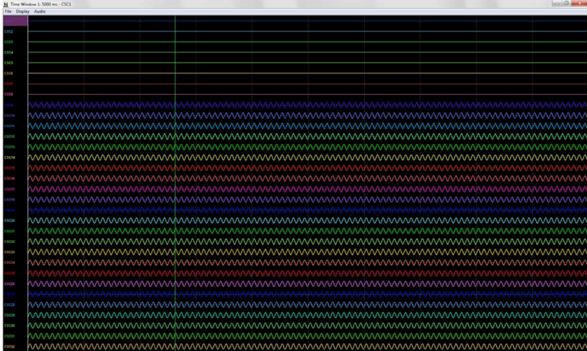
Figure 4-3 Bank 2, 3 and 4 Switches Up. Bank 1 and Reference Switches Down. Switch the Bank 2 Switch to the Ground Position (Down). Observe the 32 CSCs. CSCs 1-16 should now be flatlined while CSCs 17-32 still show a reduced (roughly 1mV PP ) version of the Minirator output. Refer to the figure below.
