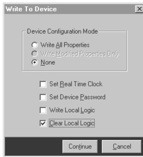
Figure 6-15. Clearing Local Logic from an RTU
