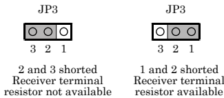
Figure 5.2. Terminal Resistor Settings
