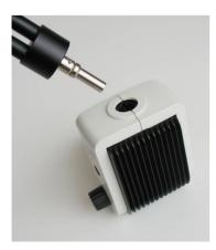
The light guide is inserted into the light guide socket as far as the stop (1). To ensure a tight fit and optimum illumination the groove must click into the retaining slot.
