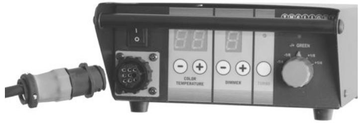
Connect the same way the female connector located at the other end of the extension cable in the input male plug coming out from the lamp head.
