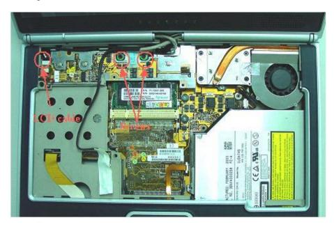
Figure 5-10 Two Screws and one LCD cable
