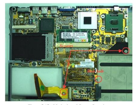
Figure 5-15 Motherboard Screws Location
