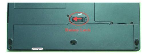
Figure 5-2 Removing the battery pack
