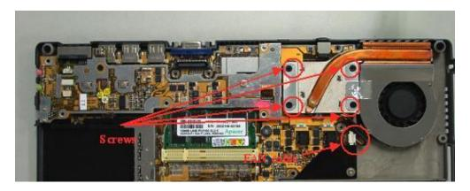
Figure 5-11 Removing Heat Sink and Sub-board
