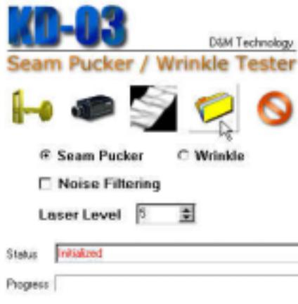
Click the save button with a folder shape, a standard MS windows dialog for file save automatically appears, and save an image file with a specific file name.
