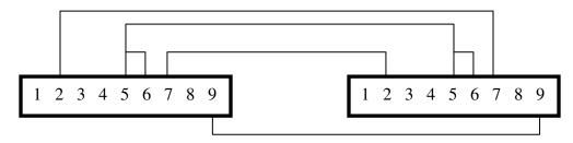
The "OUT" program function sets the logic level of pin 5. Pin 5 of both pumps is attached to pin 6 of both pumps. Therefore, if either pump disables Pump Control, then Pump Control will be disabled on both pumps. Attaching pins 2 and 7 to each other synchronizes starting and stopping of the pumps. If either pump starts or stops, then the other will start or stop.
