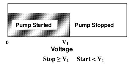
Sets a trigger voltage at which the pump will stop.
