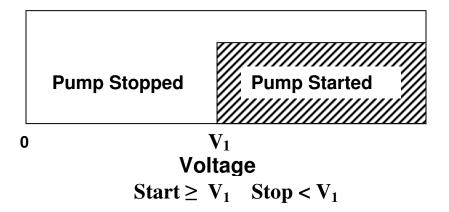
Sets a trigger voltage at which the pump will start.
