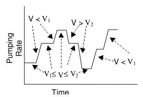
Adjusts the pumping rate to maintain a voltage window, such as from a pH meter or pressure meter. For example, as the pH increases above the  $V_2$  voltage level, indicating high pH, the pumping rate decreases by  $\Delta R$  to lower the pH. Below the  $V_1$  voltage level, indicating low pH, the pumping rate will increase to raise the pH. Between the  $V_1$  and  $V_2$  voltage window, the pumping rate will be held steady.
