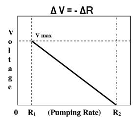
Ramp up or down the pumping rate with the Voltage. The pumping rate will be proportional or inverse proportional to the input voltage. The pumping rate will be updated 5 times a second.
