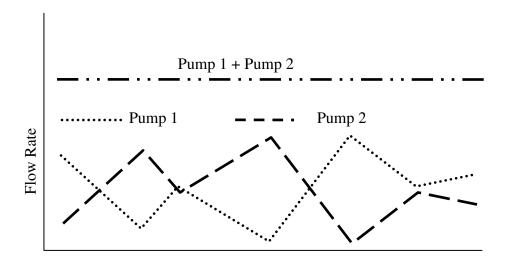
Create a closed loop, constant flow rate system, which can vary the concentration of a chemical in reaction to a sensor, such as a pH meter or pressure meter.
