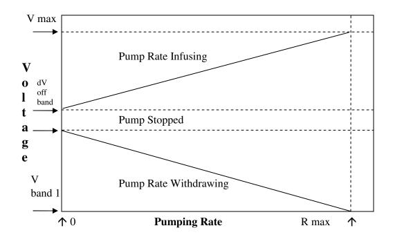
Permits a joystick type of device to be used to control the pump speed and direction. Pushing forward from the central position will start the pump infusing, starting slow, and then increasing in speed. Pulling backward from the central position will start the pump withdrawing, starting slow, and then increasing in speed. The neutral central position will stop the pump.
