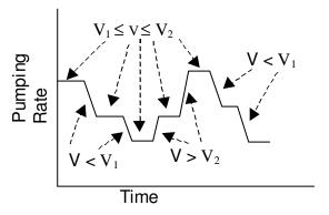
Adjusts the pumping rate to maintain a voltage window, such as from a pH meter or pressure meter. For example, as the pH increases above the  $V_2$  voltage level, indicating high pH, the pumping rate increases by  $\Delta R$  to lower the pH. Below the  $V_1$  voltage level, indicating low pH, the pumping rate will decrease to raise the pH. Between the  $V_1$  and  $V_2$  voltage window, the pumping rate will be held steady.
