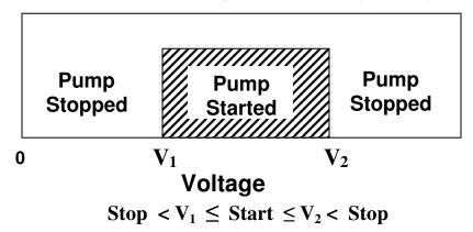
Sets a voltage trigger window within which the pump will start. Outside the voltage window, the pump will be stopped.
