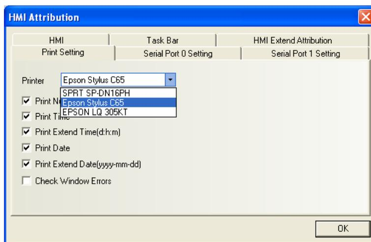
MT5000/4000 supports the connection with EPSON ESC/P2 printers or other compatible printers.
