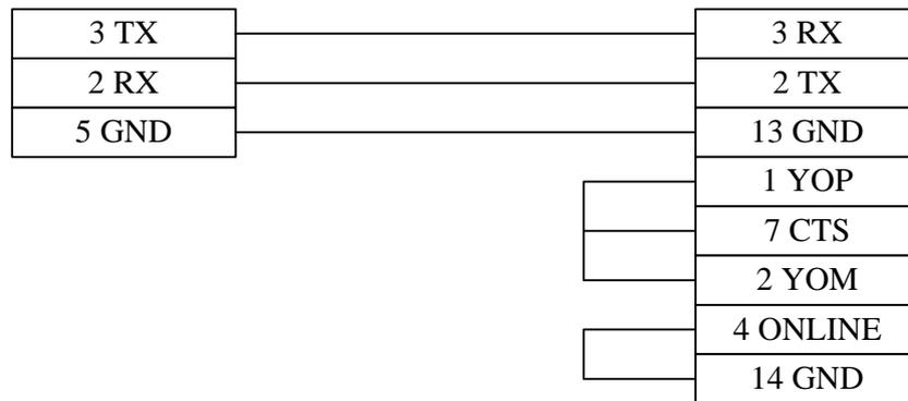
5. CPU (DL430/DL440/DL450 CPU Port1 & DL350 CPU Port2 RS232)
