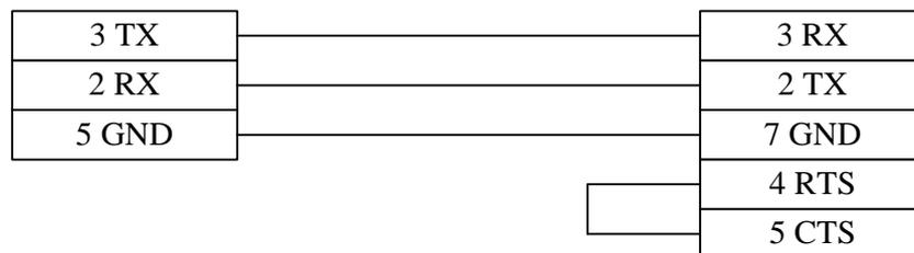
**6. CPU (DL430/DL440/DL450 CPU Port1 & DL350 CPU Port2 RS422)**
