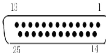
The MT5000 series and the MT4400T/MT4500T series provide a printer interface. The interface setting is the same as a PC interface. The MT4300 series provides a 15-pin print interface.
