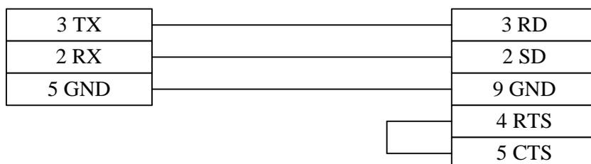
5. Communication module (C200HW-COM03/06 communication module RS 422)
