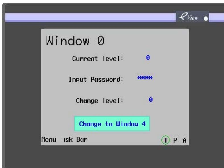
Enter 1 in the (**Change Level**) frame, but the current level will not change to 1 because it is not permitted to change a window with a lower security level to a window with a higher security level, as shown below:
