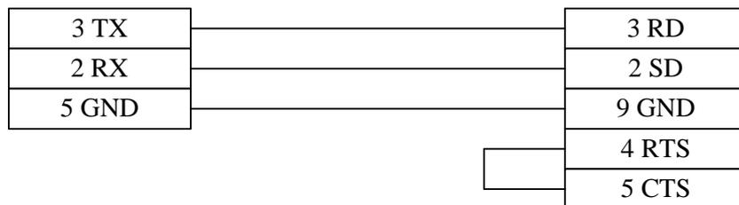
**Note:** The following CPUs can be connected with the touch screen directly: CQM1-CPU21/41/42/43/44 and CQM1H-CPU21/51/61. For hardware settings, refer to the technical manuals provided by OMRON.
