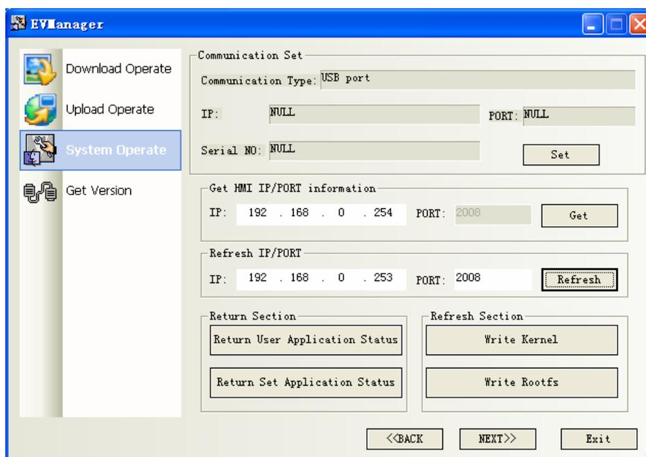
**Note:** To obtain IP/update IP address, the user can only select the communication mode of serial port or USB.
