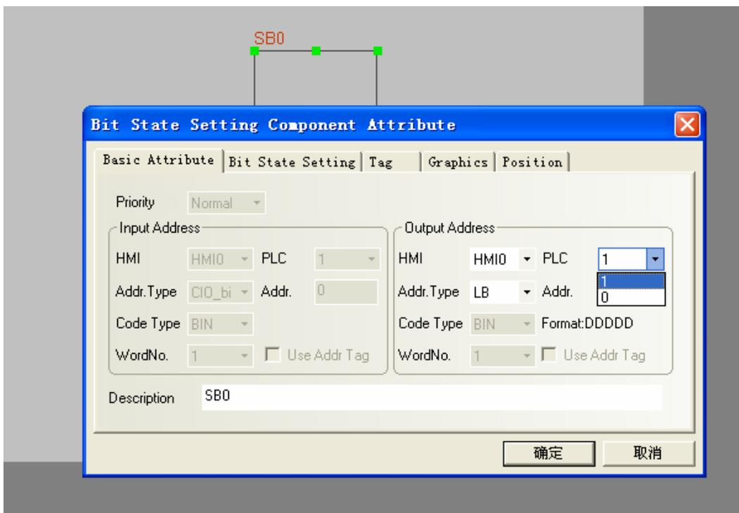
Place a bit setting component, set the PLC No. to 1, and select OMRON address for address type.
