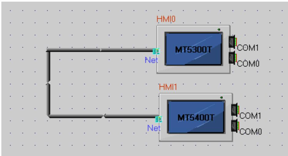
Lead another Ethernet cable from **Communication Connection** and connect it to the Net interface of a touch screen. In this way, three touch screens are connected, as shown in the figure below:
