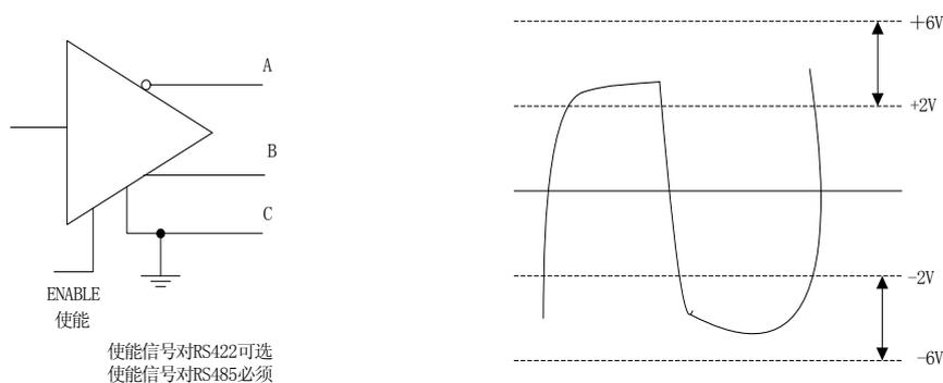
Corresponding specifications are made for the receivers. AA and BB are connected with balanced twisted pairs between the transmission end and the receiving end. When the level between AB at
