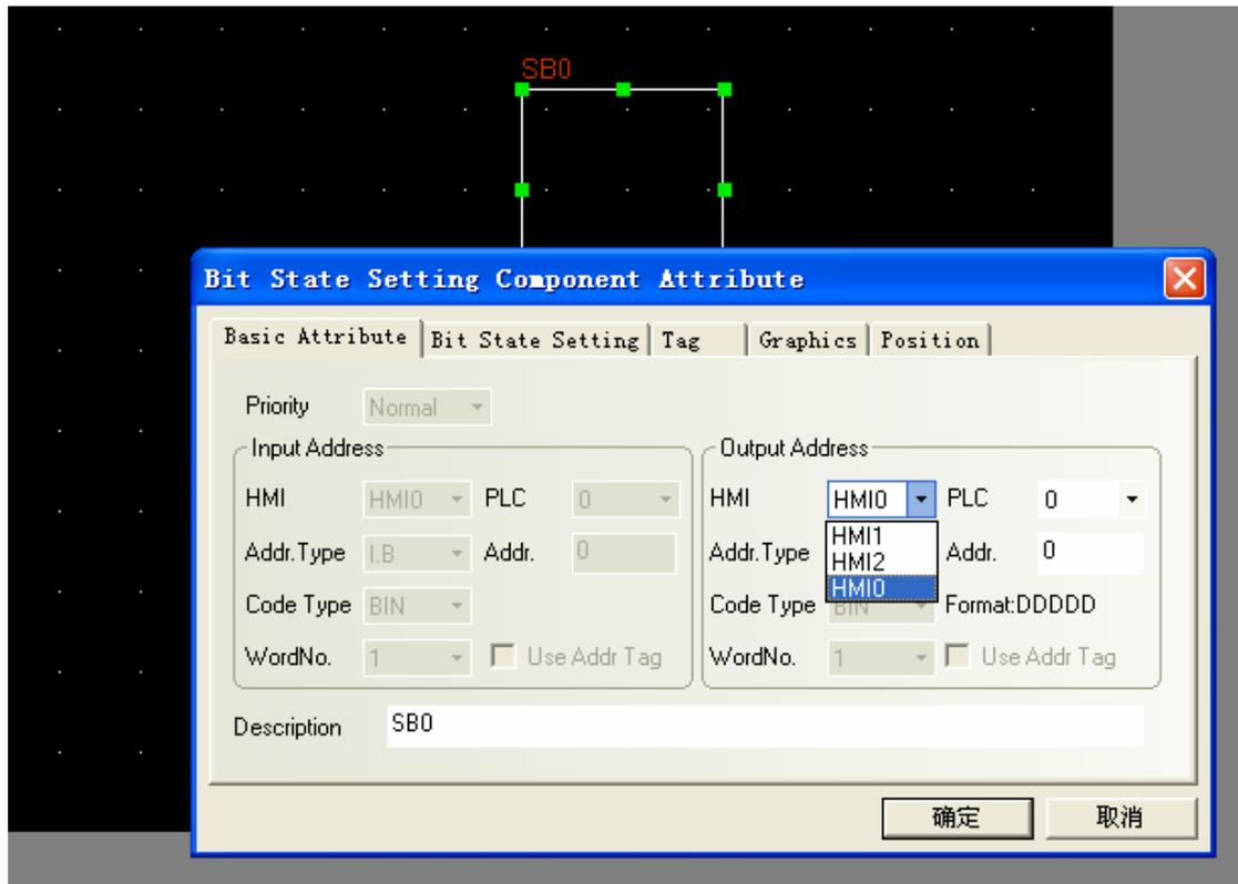
Compile the component, select the **(Offline Simulation)** mode, select the corresponding touch screen number, and click **(Simulate)** to perform offline simulation.
