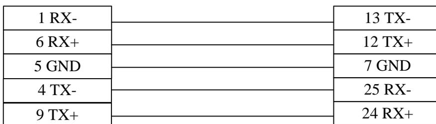
**8. Data communication unit (D2-DCM module of DL205 series, D4-DCM module of DL405 series, RS232)**
