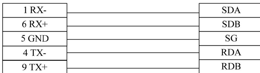
**Note:** Only K200S CPU K3P-07BS provides built-in RS-422/485 port. Set the PLC type to LG MASTER-K Cnet, and pay attention to the setting of communication parameters.
