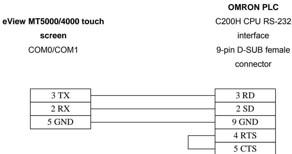
**Note:** The wiring method of SRM1 series PLCs is the same as that shown in the above figure. In the CPUs of the C200H series PLCs, there are Dial in-line Package (DIP) switches for parameter setting. Please pay attention to parameter settings. For detailed hardware settings, refer to the technical manuals provided by OMRON.
