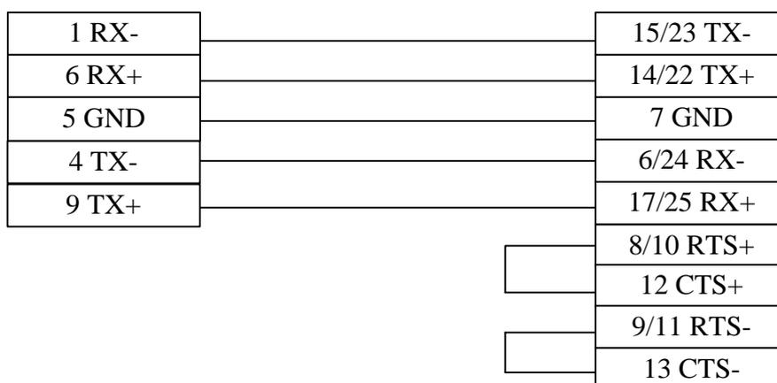
**Note:** Among all PLCs in the DL205 series, only DL240/DL250 CPU supports D2-DCM unit. All PLCs of the DL405 series support D4-DCM unit. Please pay attention to the settings of the DIP switch. It must be set to the DirectNET Slave mode. In addition, pay attention to the setting of the
