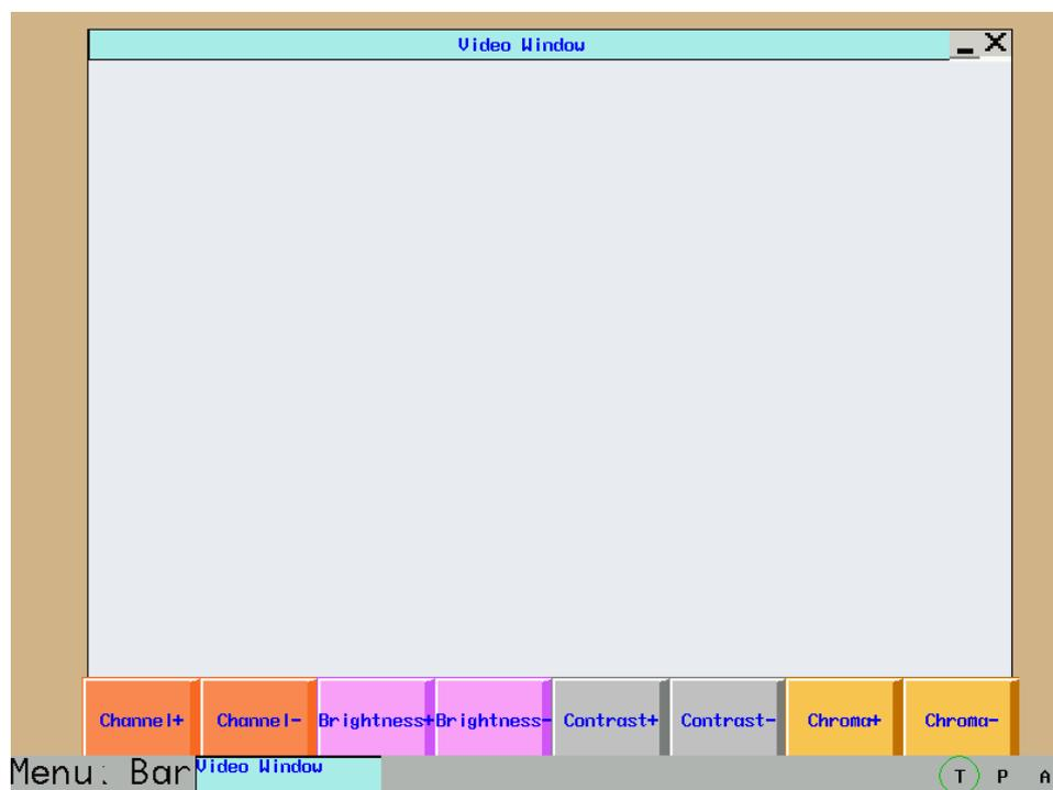
Install a camera properly, download the project to the HMI, click **[eChannel+/Channel-]** to
