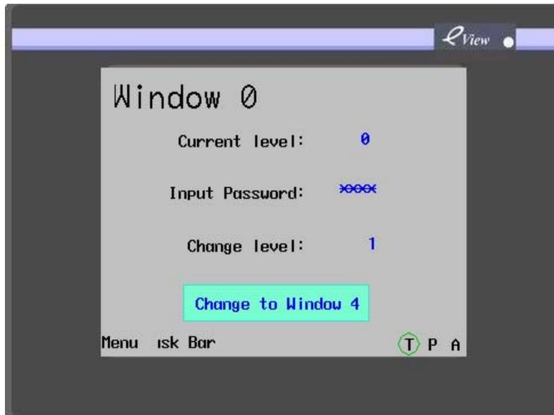
Then, enter the password **1111** to change the current security level to 1, as shown in the figure below:
