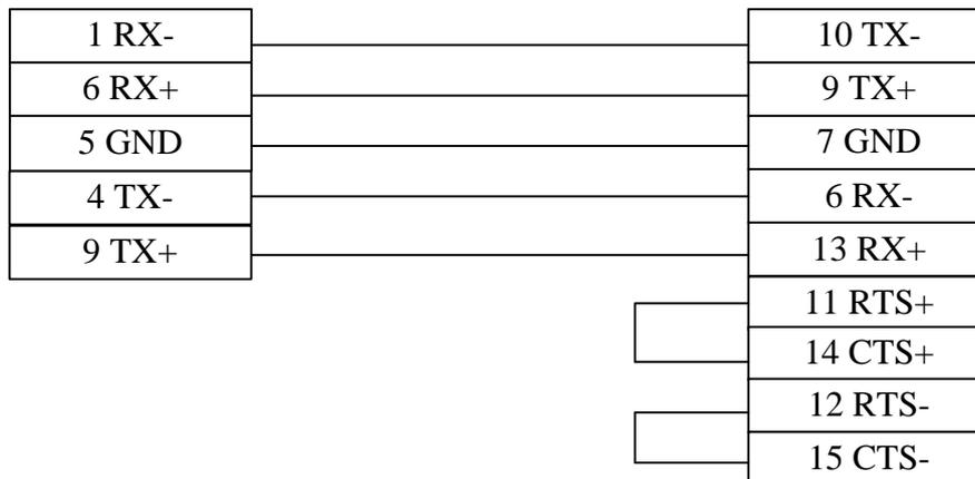
**Note:** Port2 of the DL250 CPU combines RS-232 electrical interface and RS-422 electrical interface. Please pay attention to the setting of the type during use.
