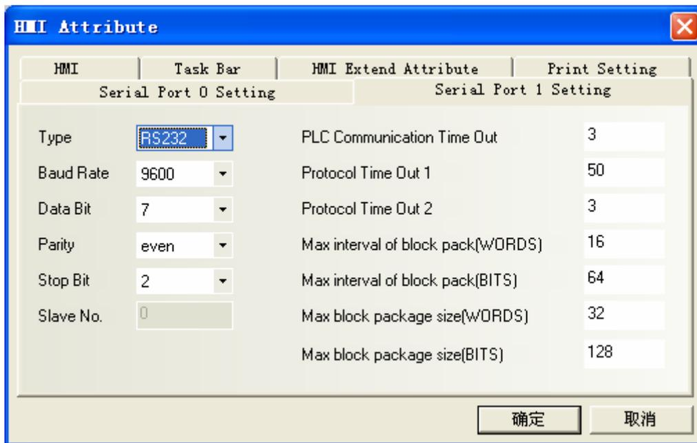
Double click the OMRON PLC and set the PLC station No. to the default value 0, as shown below:
