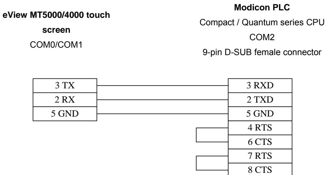
**Note:** Modbus serial ports of the CPU A984 and E984 241/245/251/255 of the Compact series, and the Modbus serial ports of the Quantum 140CPU series are all 9-pin RS-232 hardware interfaces. Where, A984-131/141 and E984-241/251 of the Compact series and the 140CPU 434/534 of the Quantum series have two Modbus ports. The wiring diagram is shown in the above figure. For related software and hardware settings, refer to the technical manuals provided by Schneider Electric.
