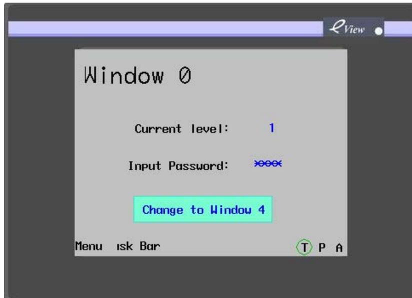
The current security level is now 1. Press the (**Change Window 4**) button, and the system successfully switches to window 4, as shown in the figure below:
