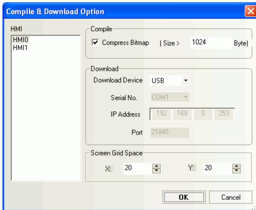
(4) If the Ethernet interface is used to download the program, the IP address should be set to be different from that of the PC. To modify the IP address, you may turn the two DIP switches in the rear of the touch screen to “ON”, and then reset the HMI to enter the built-in SETUP window.
