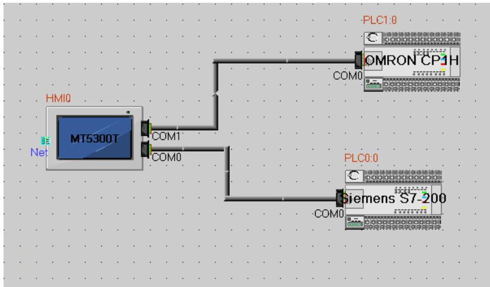
One MT5300T touch screen, with COM1 connected with a Siemens S7 200 PLC and COM0 connected with an OMRON PLC.
