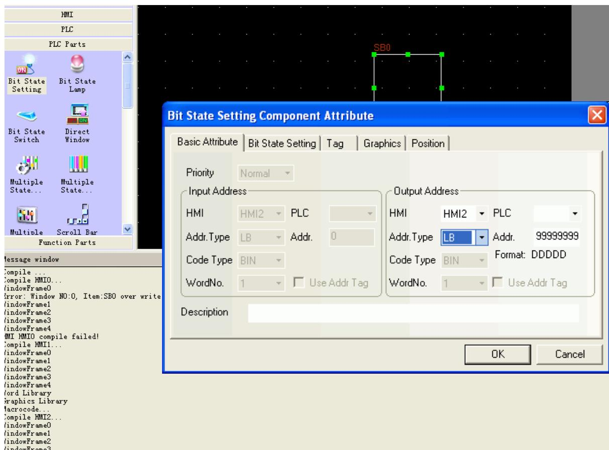
Refer to Chapter 14 for address range of PLC components or refer to related PLC data to modify the PLC component address.
