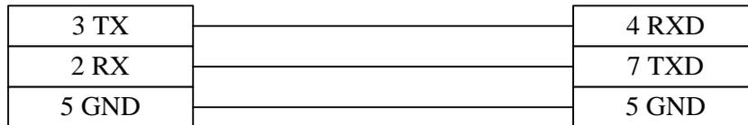
**Note:** When the Cnet communication mode of K80S/K200S/K300S/K1000S is used, set the PLC type to LG MASTER-K Cnet. The setting of communication parameters must be consistent with that of the touch screen.
