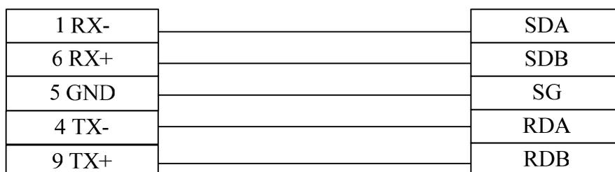
**Note:** C200HW-COM communication module supports only the C200H ALPHA series of CPUs. Pay attention to the settings of DIP switches. For hardware settings, refer to the technical manuals provided by OMRON.
