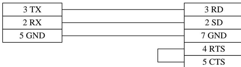
**Note:** Please pay attention to the setting of four DIP switches on the module. For indications of these DIP switches, refer to the technical manual of communication modules of OMRON. The wiring method of the CPUs of the C series PLCs developed at an earlier stage, like C20H/C28H/C40H CPU, is the same as that shown in the above figure.
