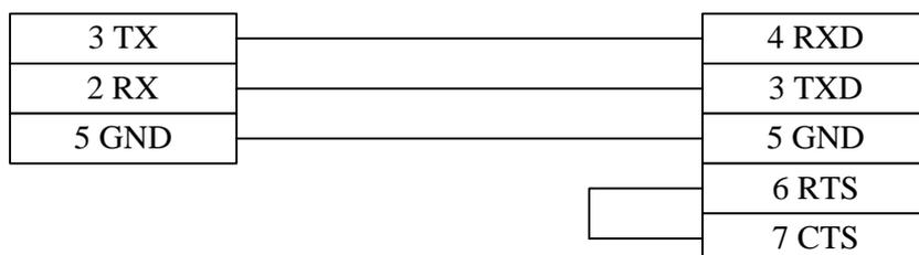
**Note:** Two Modbus serial ports of the CPU E984 – 258/265/275/285 in Compact series and the COM1 of the CPU 171 CCS 700/760/780 in the Momentum series are all RJ-45 hardware interfaces. The wiring diagram is shown in the above figure. For related software and hardware settings, refer to the technical manuals provided by Schneider Electric.
