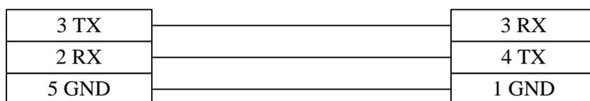
**Note:** Port1 & Port2 of the DL05 series, Port1 & Port2 of the DL240 series, Port1 of the DL250 series, Port1 of the DL350 series, and Port2 of the DL450 series are all RJ-12 hardware interfaces. The wiring method for them is the same as that shown in the above figure. Please note that the address of some ports is 1 invariably, but the address of some other ports has to be set. Make sure the communication protocol of the port is set to K sequence.
