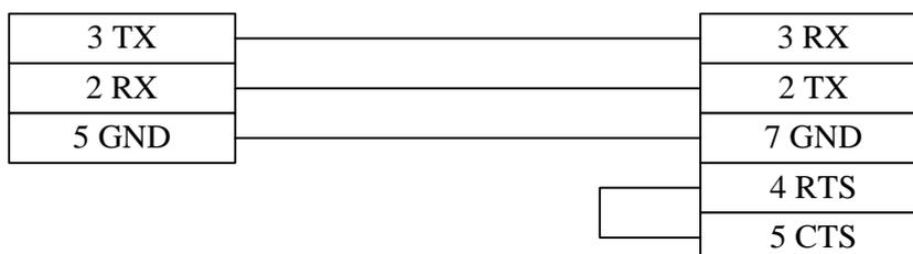
**Note:** Port2 of the DL250 CPU combines RS-232 electrical interface and RS-422 electrical interface. Please pay attention to the setting of the type during use.
