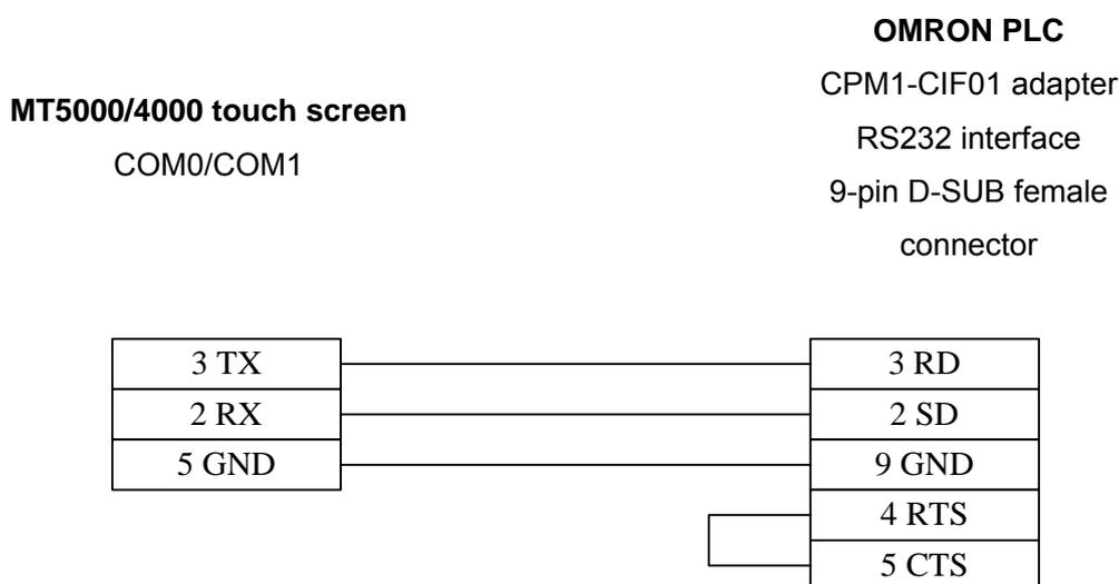
**Note:** Set the mode setting switch of the CPM1-CIF01 adapters to the Host Link communication mode.
