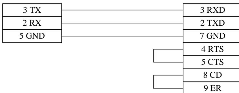
**Note:** In the FP1 series, only FP1-C××C models support 9-pin RS-232 interfaces. The tool port of the FP10SH can also be used to connect with the touch screen. The wiring method is shown in the above figure.
