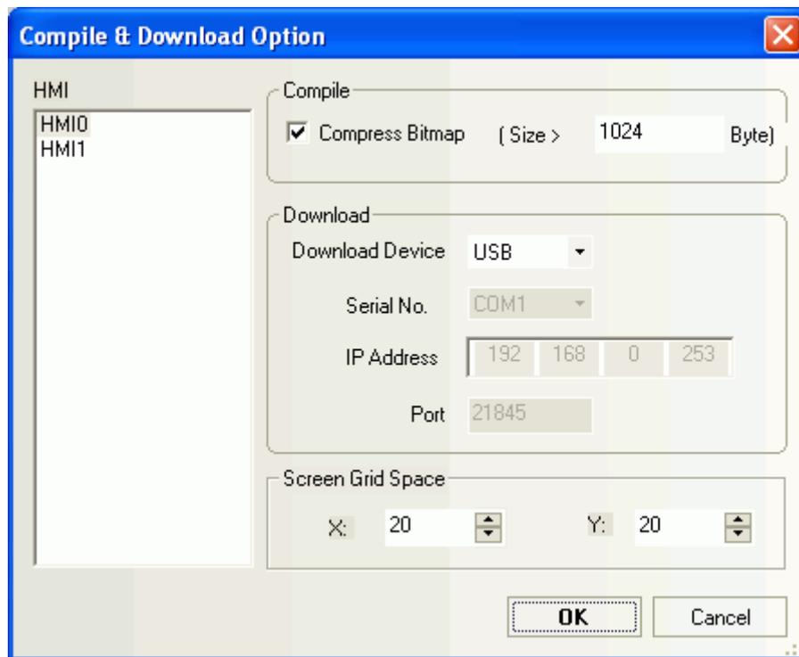
A USB cable is included in the package of MT5000/4000 panel. Connect MT5000/4000 panel to the USB port of the PC with that cable before download.
