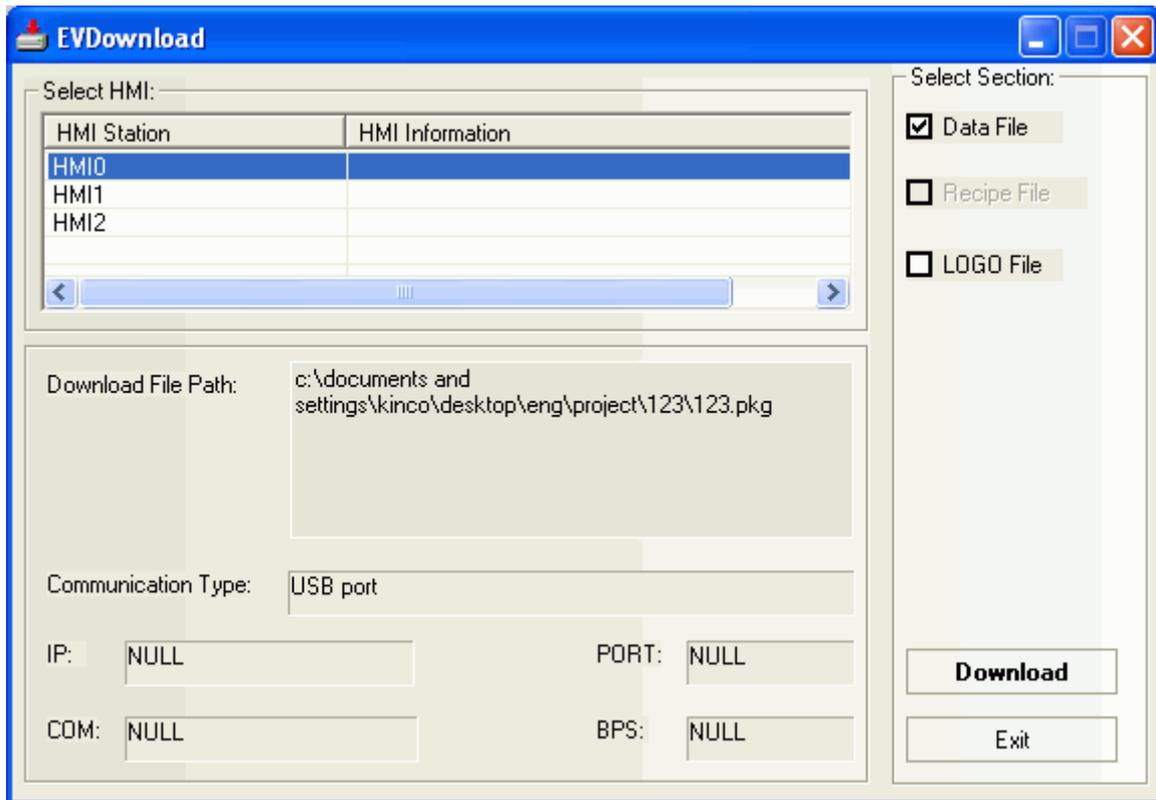
Downloading between different touch screens must be conducted via a PC. Firstly, upload from a touch screen to the PC and then download from the PC to another touch screen.
