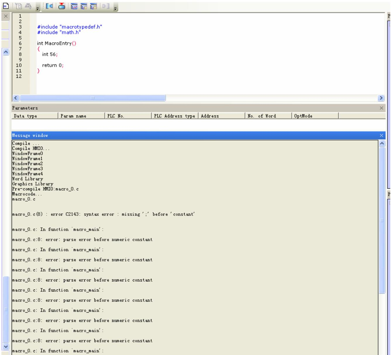
The screenshot displays a software development environment with a code editor and a message window. The code editor shows a C macro definition for `MacroEntry()` with a syntax error on line 8. The message window shows the compilation process and the resulting error messages.
