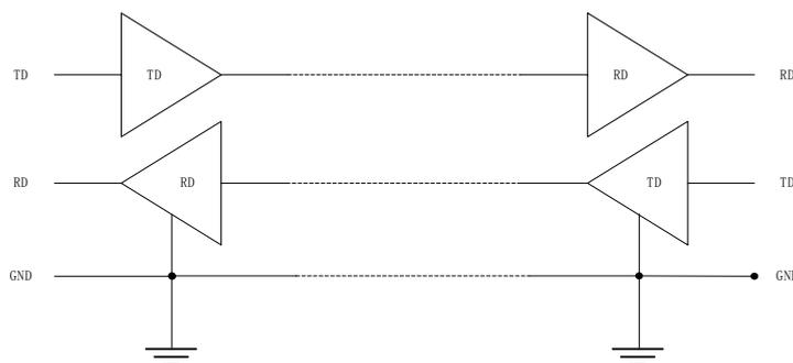
Since RS-232 adopts the full-duplex transmission mode, it has independent transmission (TD) and receiving (RD) signal cables and a grounding signal cable. The purpose of CTS and RTS is intended for handshaking control between the eView MT5000/4000 and the PLC. The CTS or RTS of only a few PLCs must be controlled by the eView MT5000/4000.
