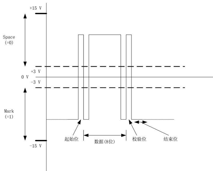
In general, logic 1 (MARK) = -3V ~ -15V, logic 0 (SPACE) = +3 ~ +15V, and each data frame (7 or 8 bits) consists of a high-voltage start bit, a low-voltage stop bit, and a parity bit. The **Bits Per Second** of data usually consists of 9600 Bit/S, 19200 Bit/S, 38400 Bit/S or 115200Bit/S.
