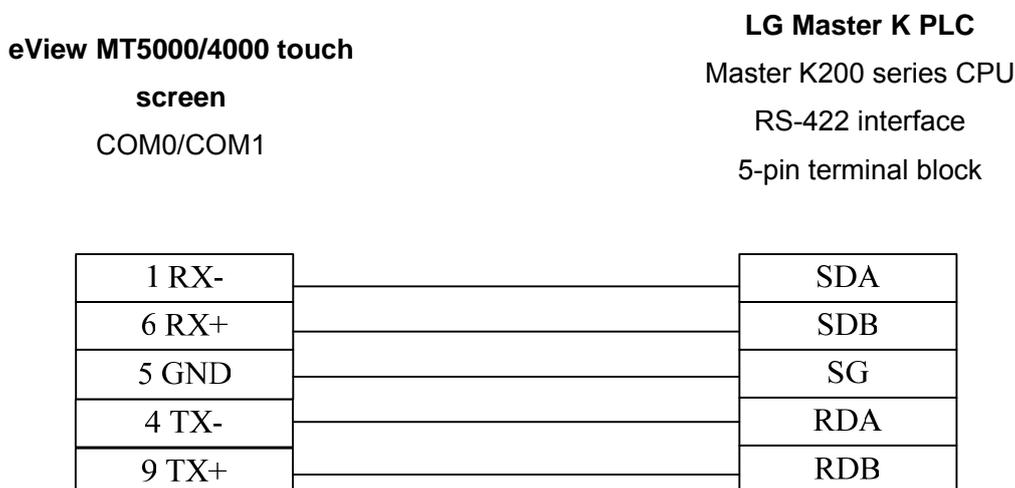
**Note:** When the Cnet module is used, the PLC type must be set to LG MASTER-K Cnet. Pay attention to the setting of communication parameters. It is necessary to use the Cnet Frame Editor software provided by LG to set the parameters. Set the mode switch on the communication module to position 3.
