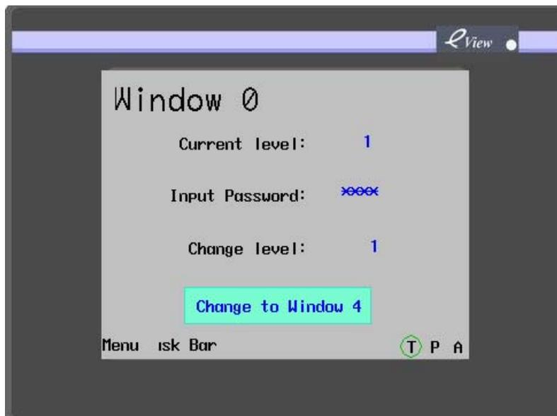
Press the function key, and the system changes to window 4. If the user enters the value 0 in the **(Change Level)** frame, the current security level changes to 0 immediately, and then, the system cannot switch to window 4, as shown in the figure below:
