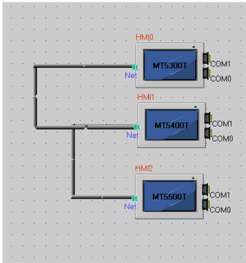
Connect the PLC with the corresponding touch screen, as shown in the figure below:
