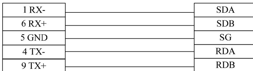
4. Communication module (C200HW-COM02/03/04/05/06 communication module RS 232)
