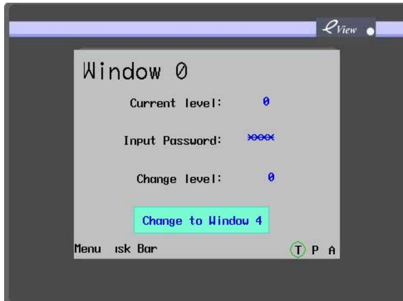
The design of different passwords for different security levels assigns different operation authorities to different operators, which enhances the security of the application system.
