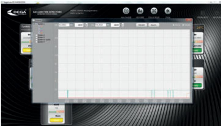
To be easily distinguished the individual sensors are shown in different colours. By setting the appropriate time intervals, we can observe the behaviour of the detection system over time.
