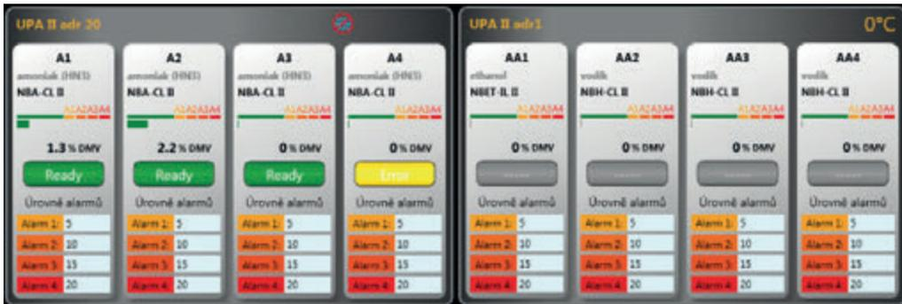
The figure in the example is showing that the detection system is composed of two UPALII controllers, each of which has four transmitters. The status and values of the transmitters are displayed, together with the alarm levels for which they are set.
