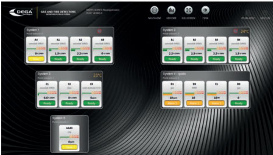
Individual objects represent the systems that consist of controllers, the transmitters of which are displayed in the systems. The number and the distribution of the systems and their controllers are dependent on the configuration of the programme.
