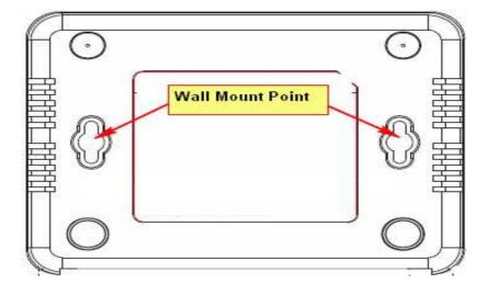
You can mount the device on the wall. There are two mounting points on the bottom of the device. Please find a proper spot where two nails can be applied. Finally, carefully mount the device onto the wall and make sure the nails are firmly locked on the mount points.
