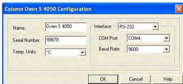
Fig. 113 Configuration window for the column oven 4050
