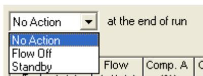
Fig. 127 Possible action at the end of run for pump S 1050 / P2.1L
