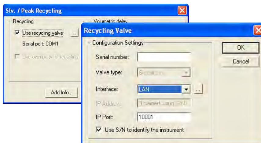
Fig. 326 Additional recycling valve setup
