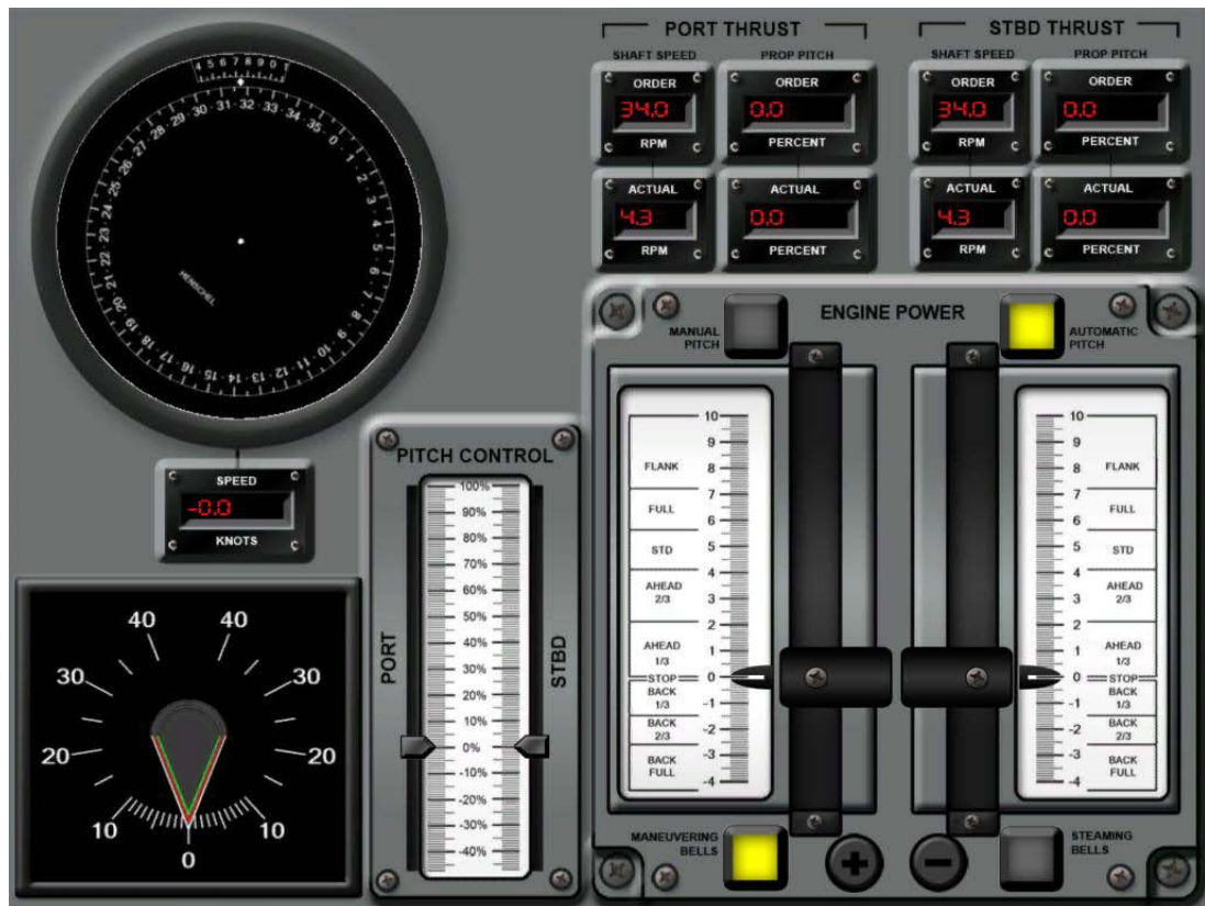
Figure 20: Large view of the touch screen throttle controls
