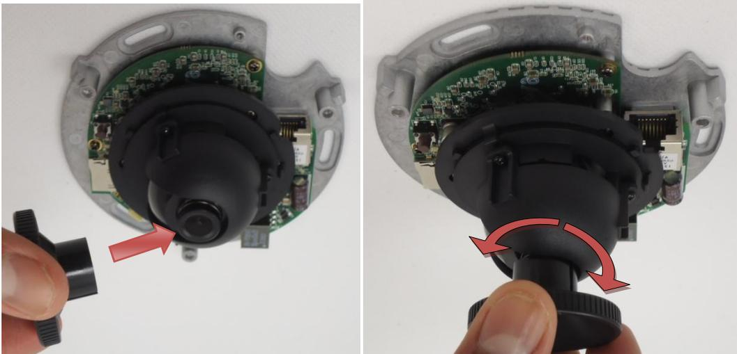
Remove the lens focus tuner.
