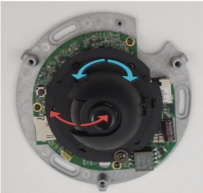
Attach the focus tuner on lens to adjust the focus of lens.
