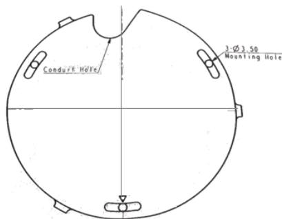
Route cables through the ceiling, taking as a reference the Conduit Hole on the drilling template. Or you may take off the removable part from the cable exit hole at the rear of the cover by sliding it out from the cover to route the cable from the camera.
