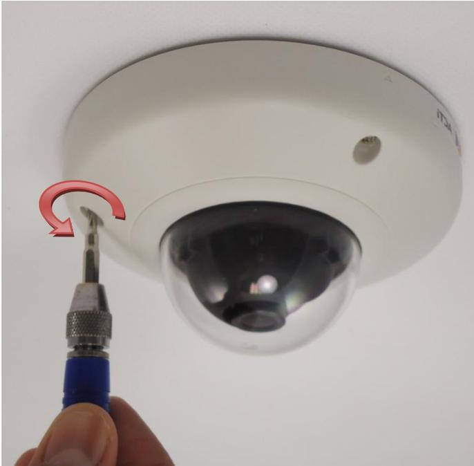
Based on the live view from the camera, adjust the viewing angle with pan and tilt direction.
