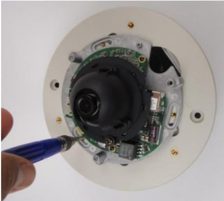
Finally, put the cover back on, and tighten with the 3 screw holes on the camera body.
