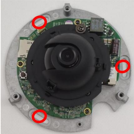
Tighten the camera body to the ceiling using the 3 screws included.
