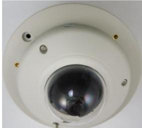
First, locate the three screw holes on the accessory that can be used to attach this camera model.
