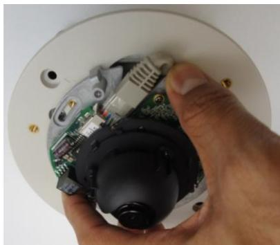
Tighten the camera body to the PMAX-0803 with the 3 screws included in the camera box.
