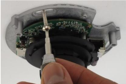
Please make sure the screw is flat on the plate, protruding is incorrect.
