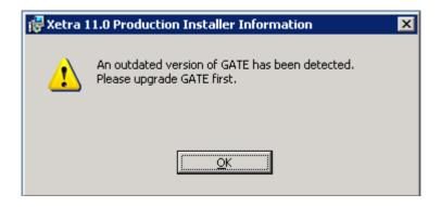
Click on <OK> and abort the installation. Then install the GATE 3.5 software as described in the "GATE Front End Installation Guide".
