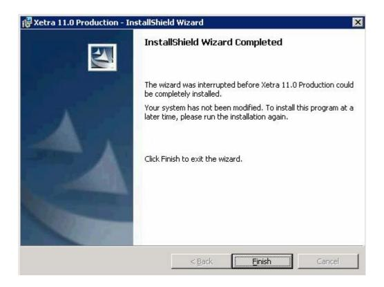
Click on <Finish> and abort the installation. Then install the GATE 3.5 software as described in the "Front End Installation Guide GATE".
