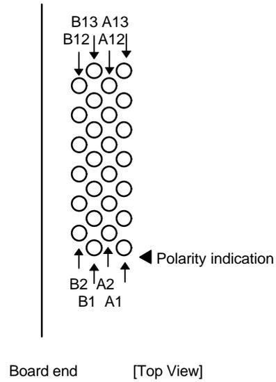
**Note** When actually arranging the pins, design them according to the connector dimensional information.
