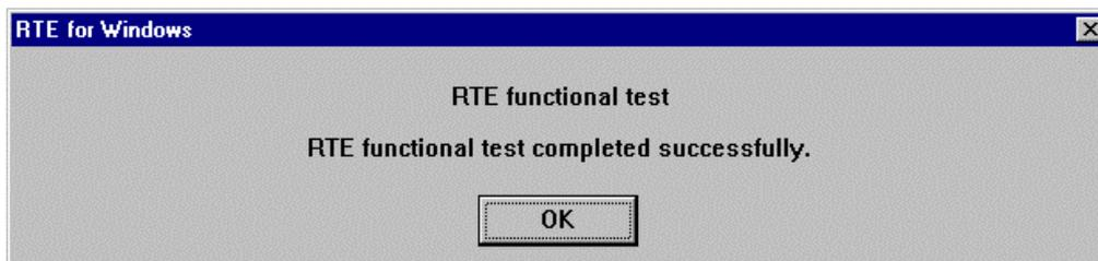
If an error occurs during the test, the N-Wire cable is not properly connected. Check its connection.
