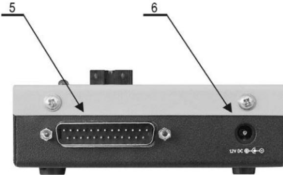
**Note:** Due to low power consumption of PREPROM-02aLV in inactive state, it doesn't require power switch.
