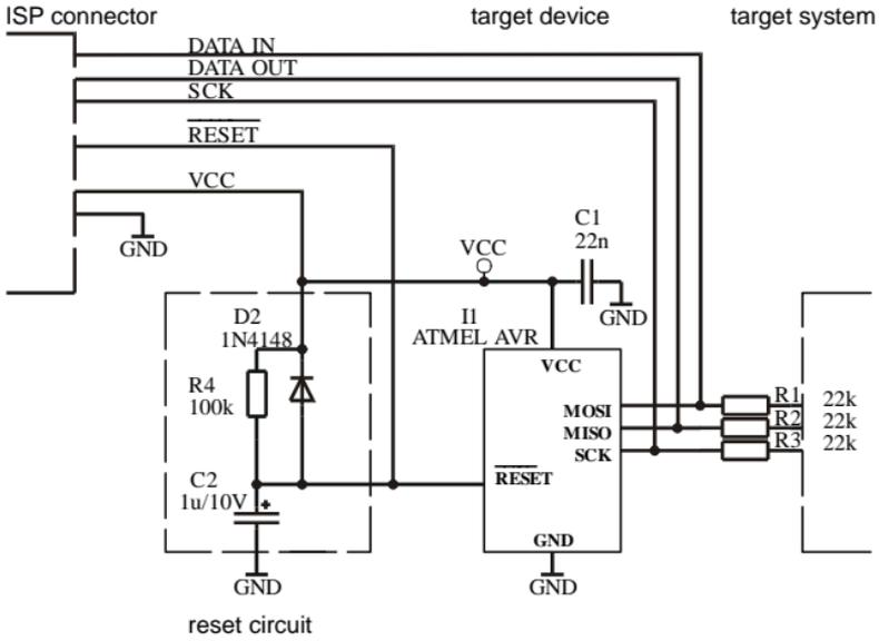
ELNEC's recommended circuit for AT89Sxxx:
