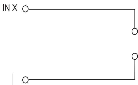
**Example wiring diagram for mode 10,11 – control button of remotely controlled relays**
