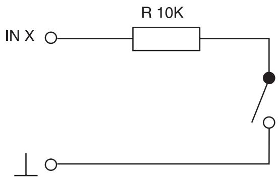
**Example wiring diagram for mode 8 – control pulse input**
