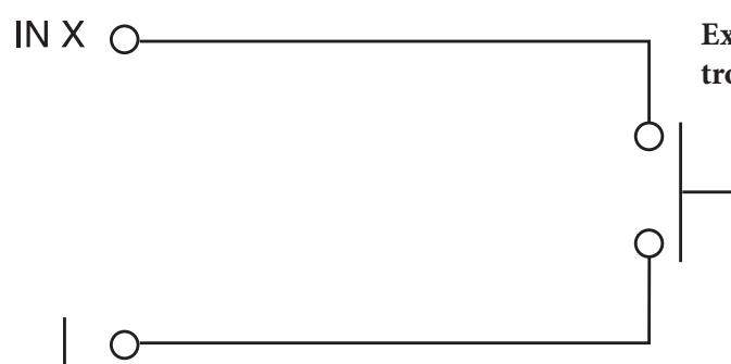
**Example wiring diagram for mode 6 - external RELAY 2 control button in flip flop mode**
