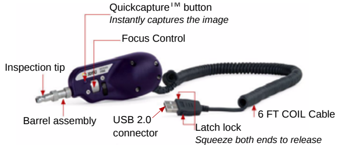
Fig. 99 P5000 Probe components
