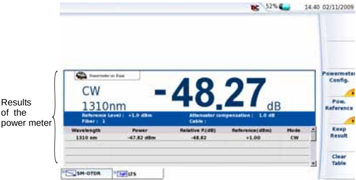
Fig. 35 Results and commands of the power meter
