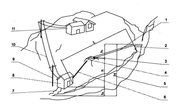
Figure 1: The project of micro hydro generator using pipe
