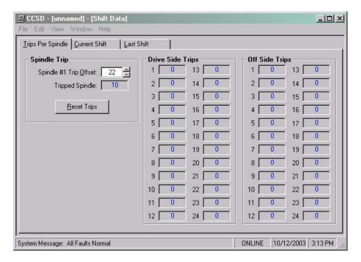
This window utilizes a "TAB" control to divide the set-up parameters into three categories, similar to that of the Keypad/Display. These sections are as follows:
