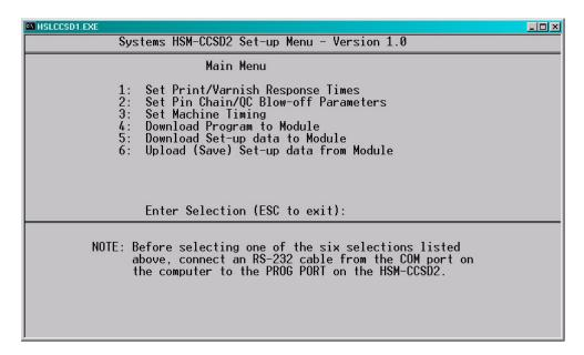
**Note:** The "HSLCCSD1" program is an on-line communications program used to interface with the M4500 module. The data displayed in the menus and set in the menus is communicated directly to the M4500. Therefore, prior to selecting any of the above selections, make sure an RS-232 cable is connected from the COM port on the computer running "HSLCCSD1" to the "PROG" port on the M4500.
