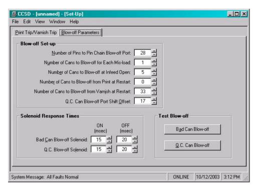
**Note:** The "Bad Can Blow-off" command button will electronically induce a mis-loaded can into the system, as well as, the "Q.C. Can Blow-off" will blow-off a can printed on spindle #1 at the QC blow-off port.
