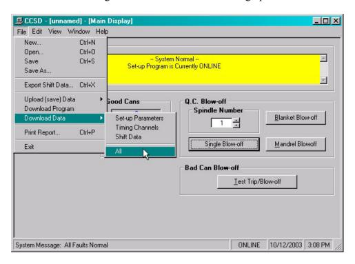
**Set-up Parameters:** This option downloads the "Set-up" data to the M4500. This includes print trip and varnish unit response times and blow-off parameters.
