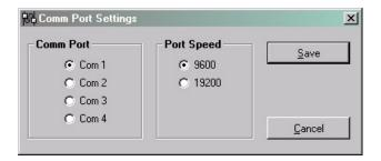
Once selected, a dialog box requesting the user to select a "Comm Port" and "Baud Rate" will be displayed. The default setting is COM1 at 9600 baud. The option to select the 19200 baud rate is to allow the user to communicate with the processor via the S4516 serial communications board.
