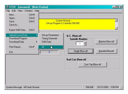
**Set-up Parameters:** This option only uploads the "Set-up" data from the M4500. This includes the print trip and varnish unit response times, as well as blow-off parameters and solenoid response times.
