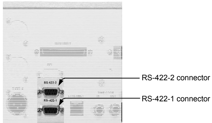
Figure 8: RS-422 Connectors – Rear Panel
