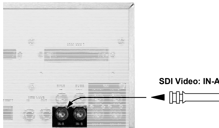
Figure 2: Video Input – V1 Rear Panel
