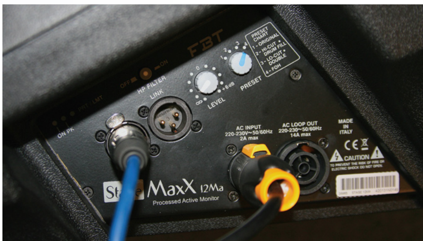
The recessed control panel houses all the audio and power inputs and outputs, as well as the input sensitivity control and four-way EQ preset selector.
