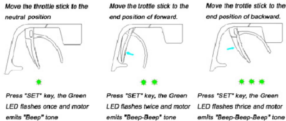
Note2: If you don't release the "SET" key after the red LED begins to flash, the ESC will enter the program mode, in such a case, please switch off the ESC and re-calibrate the throttle range again from step A to step D.
