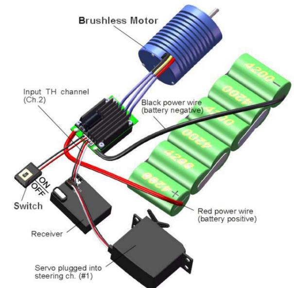
channel to the "Reverse" direction, and then the motor will run oppositely. Please calibrate the throttle range again after changing the direction of throttle channel.
