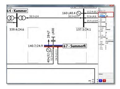
As you can see graphical representation of bus reflects parameters entered with context panel. In addition, any connected to bus object can be edited individually. At the picture below there is generator context panel, available for selected generator object.
