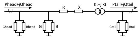
Difference is in the way of shunt part modeling. Ordinary branch with Kt=1 has shunt conductance divided equally between head and tail buses. Transformer branch with Kt=1 has whole shunt conductance at head bus.
