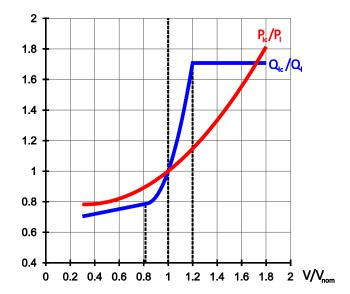
LRC on the figure on active and reactive loads is presented on the figure<sup>1</sup>. Active power LRC is modeled as single polynomial in  $\left(\frac{V}{V_{\text{max}}}\right)$  range from zero to infinity.
