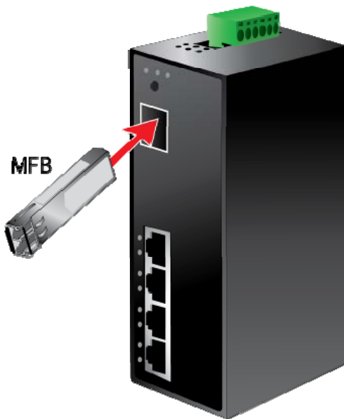
Figure 2-16 Plug in the SFP transceiver
