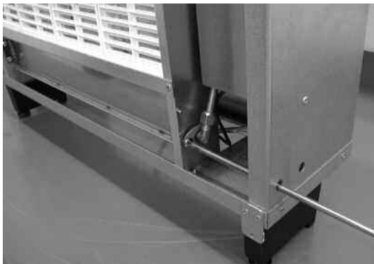
Fig. 9 Injector fixing bracket removal
