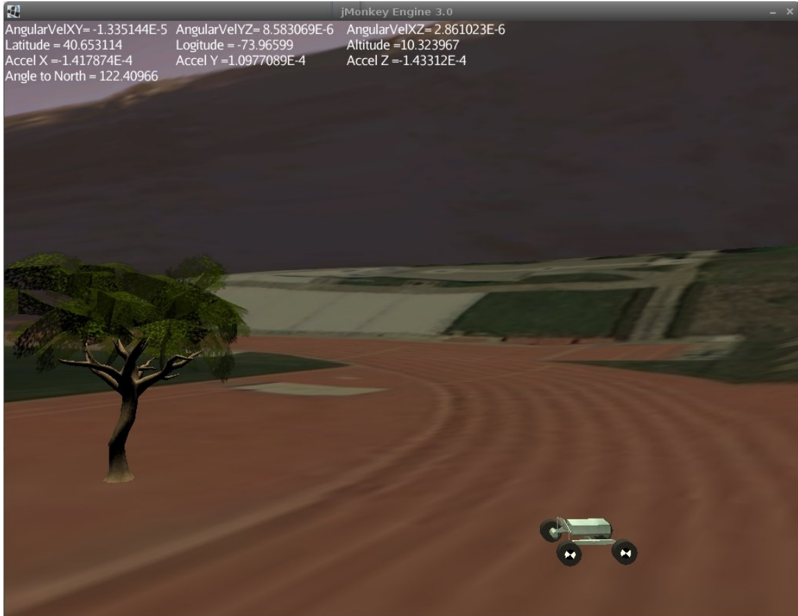
Figure 5.1.7 Simulator window showing gyroscope, accelerometer, GPS and Compass values as well as the robot vehicle model, and a tree obstacle. The terrain is from Google Earth of the track at the University of North Carolina at Charlotte.
