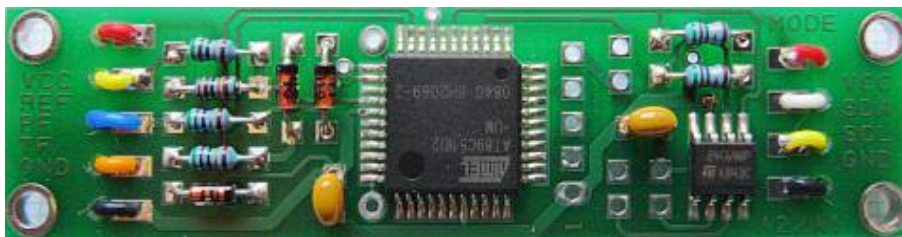
Figure 6: AVA-07-DEMO board measuring 2.75" x 0.7" (69.85mm x 17.78mm).
