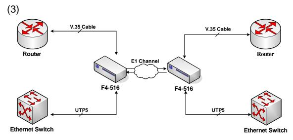
Make use of F4-516 to link routers and Ethernet switches by
