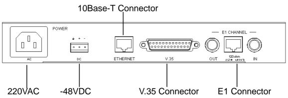
Note: 220VAC & -48VDC power input are alternative, in one device, there is only one kind of power input.
