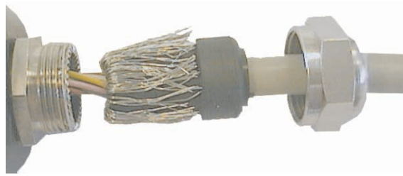
Fig. 18: Apply the shield to the PG screw of the encoder. 01948AXX
