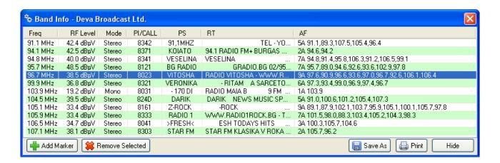
Band Info Table represents an additional information from the Analyze of the frequency band. Besides frequency, PI/CALL and PS, are shown station mode (stereo or mono), RF Level, Radio Text and AF List if during the period of peak analyze there were enough RDS data to extract AFs. By using the button Add Marker it is possible to add other frequencies. The desired frequency is selected by the Marker (See FM Band Spectrum Analyzer - 4).
