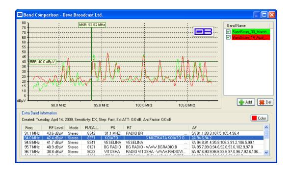
The main purpose of this tool is to provide easy way for visual comparison between different spectrum plots. The tool utilizes BND files, which are saved previously from Band Analyzer (See Band Analyzer Results Saving). The tool overlays different spectrums but is indifferent about comparison itself, which is granted entirely to user.
