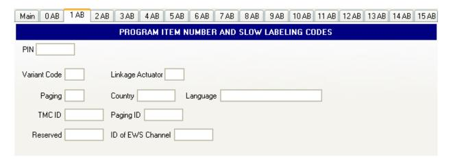
The most significant five bits in block 4 which convey the day of the month, if set to zero, indicate that no valid Program Item Number is being transmitted. In this case, if no Radio Paging is implemented, the remaining bits in block 4 are undefined. However, in the case of type 1A groups only, if Enhanced Radio Paging is implemented, the remaining bits carry Service Information.
