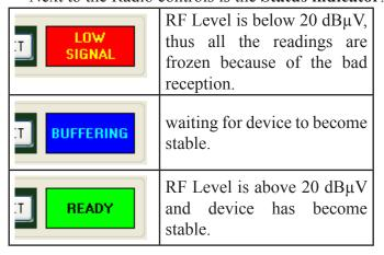
Upon changing working frequency, FM Analyzer switches to BUFFERING state and clears all collected data.
