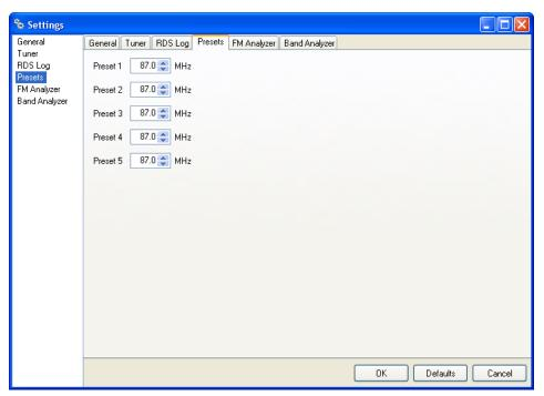
Using this feature you can assign up to 5 easy to access memory presets (See FM Tuner, Modes and Presets - 14,15). Frequencies assigned here, correspond directly to the quick preset buttons situated along with the rest of the tuner controls. Intended to serve as a quick access to 5 favorite stations, preset button needs no more than a click. Presets can be assigned from here as well as from Quick Save buttons. Saving and Recalling is very easy which explains why they are "Quick Presets".
