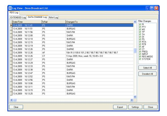
In the Data Change Log sub window are listed all occurred changes. In the right side are situated filtering options, allowing to choose which changes to be listed.
