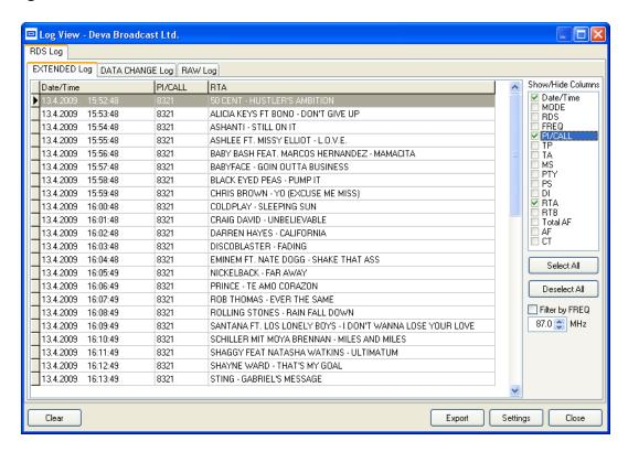
In the Extended Log sub window are listed main RDS parameters and tuner condition, saved at predefined period. In the right side are situated filtering options, allowing to choose preferred columns and frequency.
