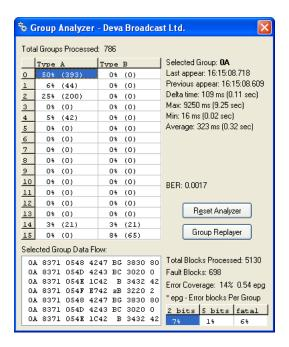
This window gives the user statistical analyze of the incoming RDS/RBDS data stream. Detailed report for the groups' quantity and ratio is included. Each group timing presence is reported in a separate table. The number of the valid or non-valid blocks processed is contained in this screen.
