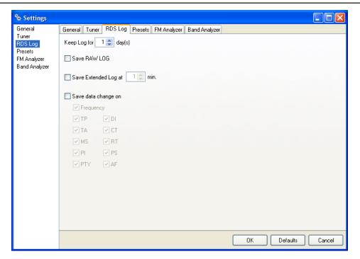
**Keep Log** – In this field you must select the length of the log in days. Maximum value: 30days. Data older than the maximum assigned period will be erased from the Log automatically.
