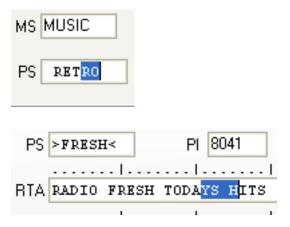
**NOTE:** In case the RDS stream is coming with errors, the "Whole PS" rule will be wrong at most of the cases, even PS may not be shown at all.
