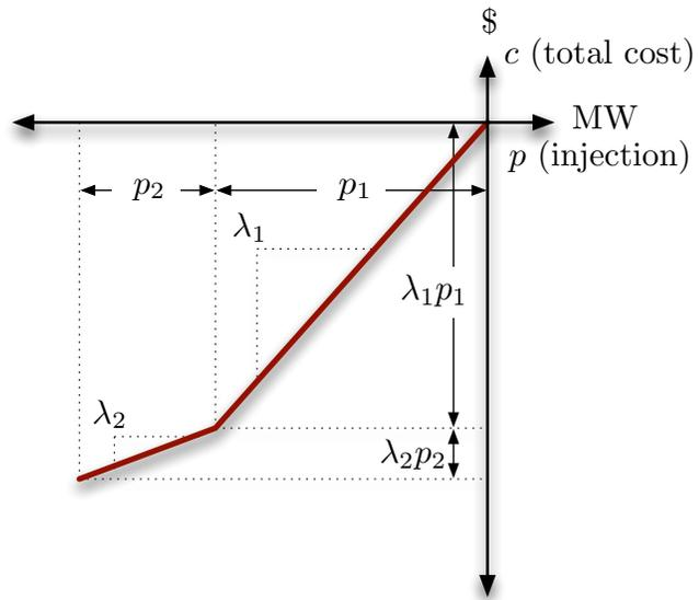
Figure 6-5: Total Cost Function for Negative Injection
