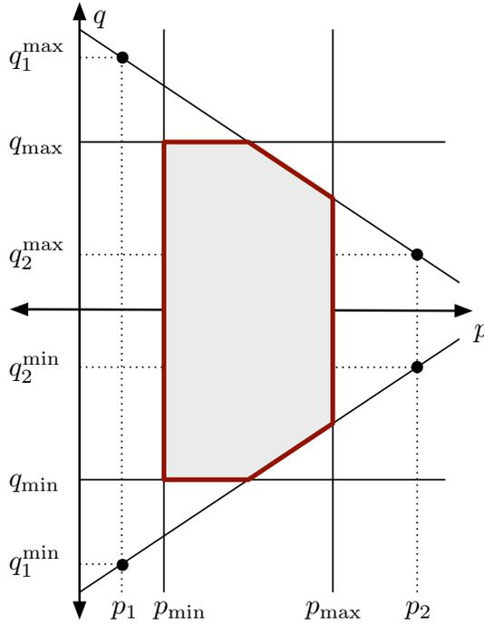
Figure 6-6: Generator  $P$ - $Q$  Capability Curve
