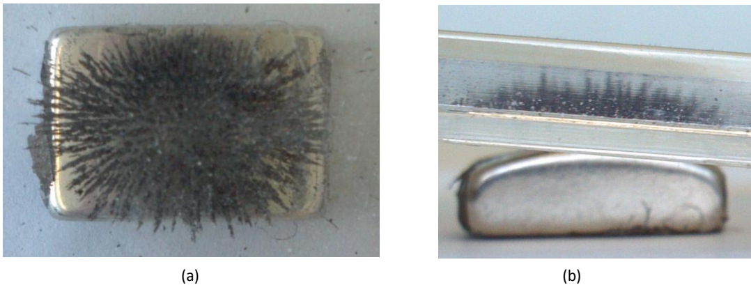
Figure 18. (a) Overhead and (b) Side views of iron filings indicating the magnetic field produced by an Air-X magnet.
