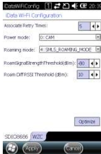
Figure 4-5 Parameter settings using the iDataWiFiConfig tool
