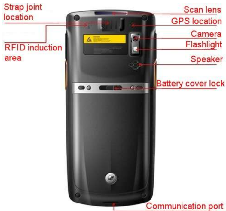
Figure 1-2 Rear view of iData 90
