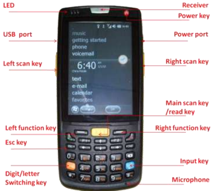
Figure 1-1 Front view of iData 90
