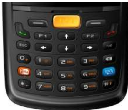
Figure 2-4 Key layout on the physical keypad
