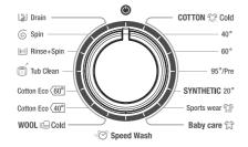
• Turn the program selector to the desired program. The indicator light of Start/Hold button is on.
