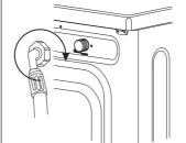
Connect the inlet hose to the water inlet valve tightly.
