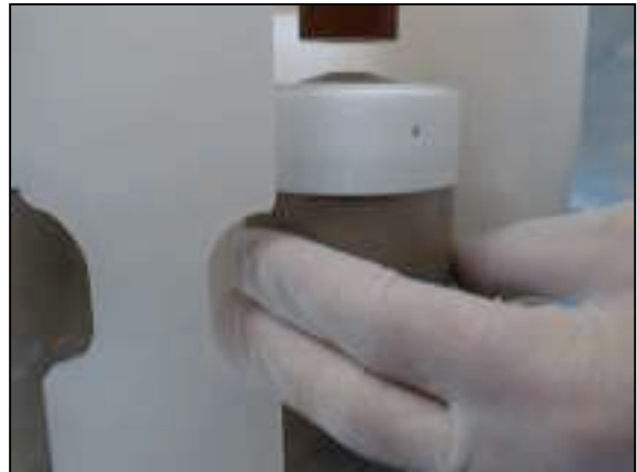
Carefully take up the vessel cover together with the TFM Teflon protection ring (picture).
