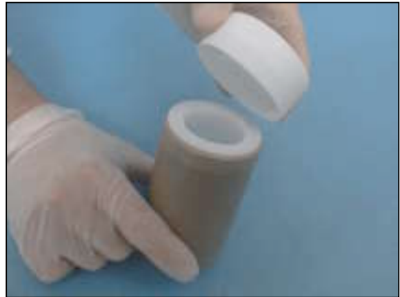
Rinse the lower part of the TFM Teflon cover with distilled water, collecting the same inside the vessel (picture).
