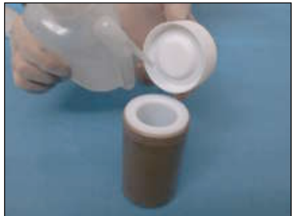
Rinse the lower part of the TFM Teflon cover with distilled water, collecting the same inside the vessel (picture).
