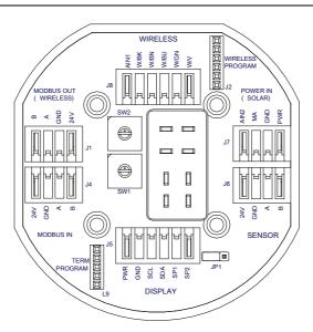
Figure 4 Model 100 Terminal Board
