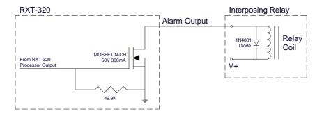
Figure 12 Internal Alarm Output Circuit
