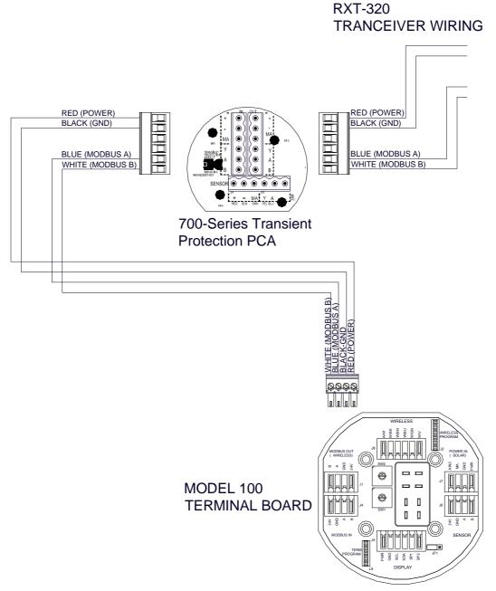
Figure 11 Wiring Diagram for Remote RXT-320 Transceiver Mounting
