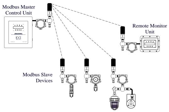
Figure 2 Typical Wireless Layout
