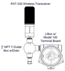
Figure 1 RXT-320 Wireless Transceiver Assembly
