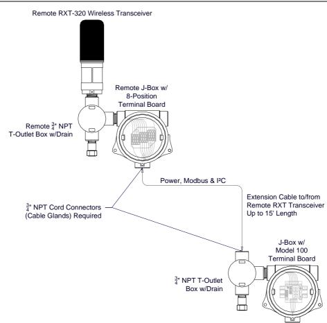
Figure 10 RXT-320 Wireless Transceiver Remote Mounting
