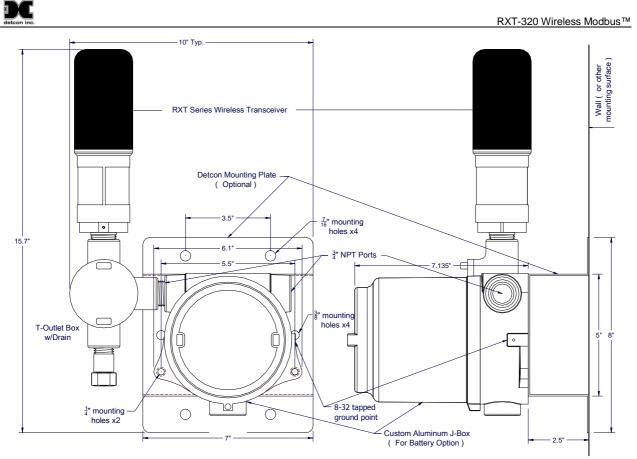
Figure 9 RXT-320 Wireless Transceiver w/Battery Assembly and Mounting Dimensions
