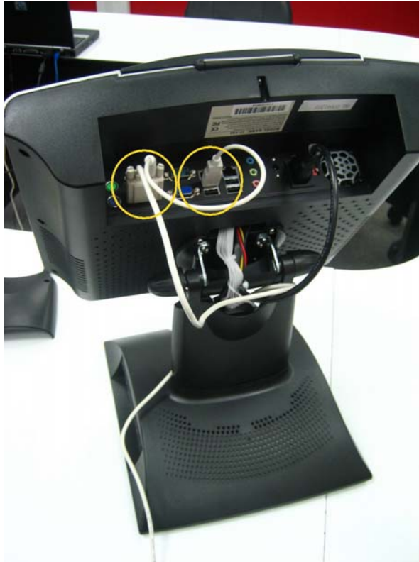
Connect RS-232 connector for data transmission and USB connector for power.
