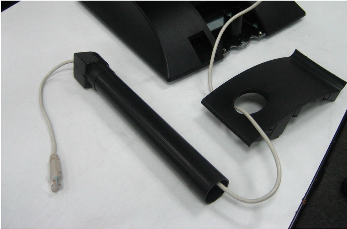
Put VFD Customer Display cable through the cover and support pipe.
