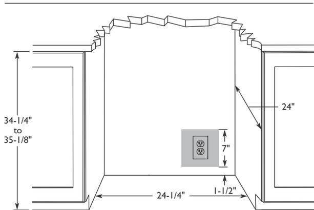
Follow the cut-out drawing The 24-1/4" width allows 1/4" for ease in installation and removal of the unit. 24" is the cabinet depth in most installations.
