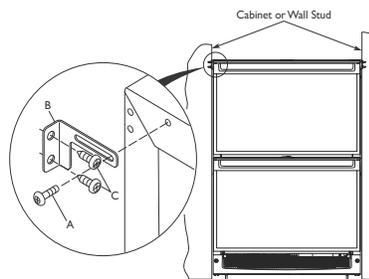
2. Insert the screws through the anti-tip bracket (B) and attach the bracket to the unit. Tighten screws securely.
