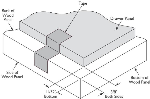
2. Place and tape the existing drawer panel on the back of the overlay panel (see above).
