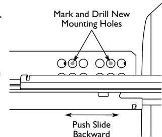
*Note:* Front location holes are shown. Corresponding rear holes will also need to be marked.
