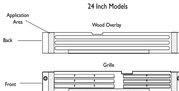
3. Carefully align the wood overlay with the grille and press into position.
