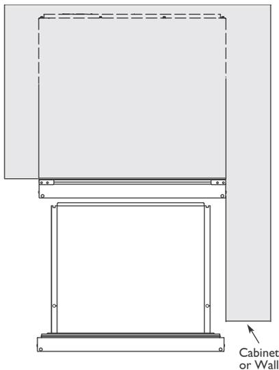
The drawer unit can be installed with an appliance or fixture located in front of it, as long as there is adequate clearance for the drawer to be opened and removed when servicing.
