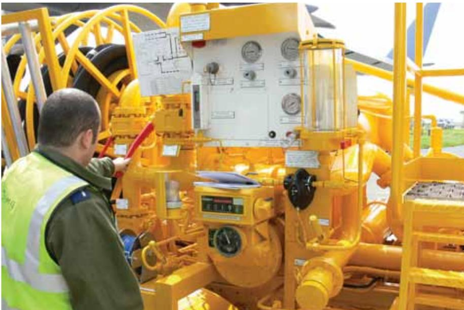
This application shows uploading fuel into an aircraft with the icountPD in use to monitor as a 'go/no go' device.
