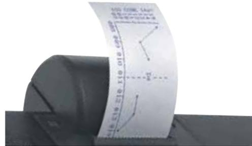
16-column printer for hard copy data. A feature of the icountLaserCM is the on-board printout data graphing option developed to support predictive maintenance procedures.
