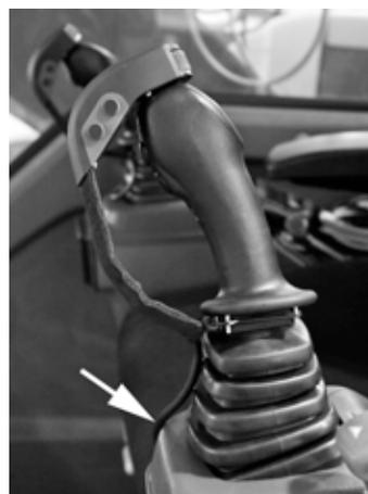
3. Position the lines so that they are not in the way of the machine operator. Make sure the lines are free of stress when the levers are pushed to their end positions.
