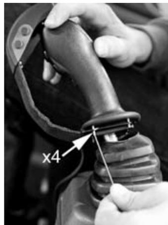
2. Mount the joysticks on the machine's levers. Position the fork of the joystick underneath the machine's control lever. Screw into place with the four screws.
