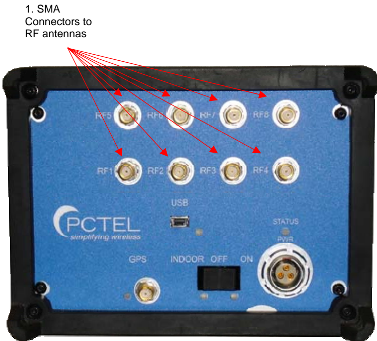
Figure 8. Connections and Switches for SeeGull MX Setup with 8 MIMO ports
