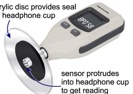
sensor protrudes into headphone cup to get reading
