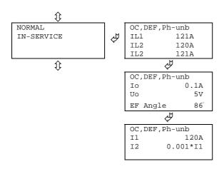
Normal display Primary value phase current 1 Primary value phase current 2 Primary value phase current 3
