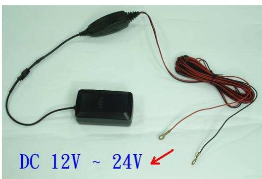
The car battery cable can be connected directly to the vehicle battery (12V or 24V) and transfer into 5V for the HI-604X. Very important: don't connect HI-604X pintail cable directly to the vehicle battery because the pintail cable takes only 5V.
