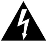
\* The lighting flash with an arrowhead symbol in an equilateral triangle, is intended to alert the user to the presence of un-insulated " Dangerous Voltage" within the product's enclosure that may be of sufficient magnitude to constitute a risk of electric shock to persons.
